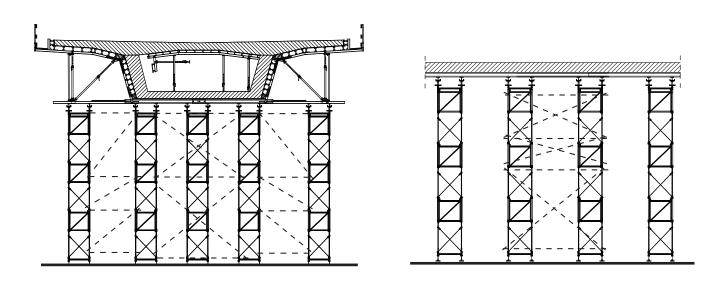
Bridge and slab construction are typical applications for ID 15*new*. Previous operational planning and preparations improve the quick and safe assembly of the ID 15*new* frame support.
