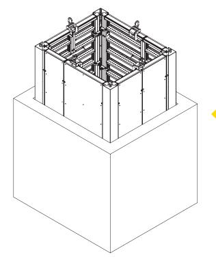
By using the mechanism of the shaft corner, the formwork can be fully released from the concrete in an instant, and it can then be lifted out by a crane in one go. It is operated from above by means of a readily accessible set-screw. No special tools are required.
